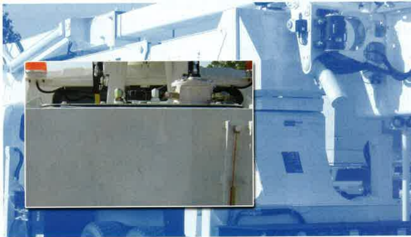
This 109-gal capacity hydraulic oil reservoir is fabricated from aluminized steel and is used in an aerial work platform bucket truck. It includes a sight gauge, filler-breather and filter
