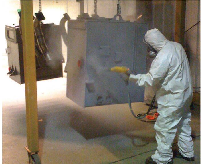
**FIGURE 6** – Tank and fill necks manufactured at The IFH Group being powder sprayed.
