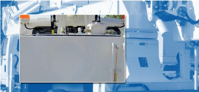
**FIGURE 5** – Reservoirs from 18 gallons to 12 gallons fabricated from aluminized steel are hot-dip-coated on both sides with an aluminum-silicon alloy to avoid the contamination problems inherent to uncoated steels.
